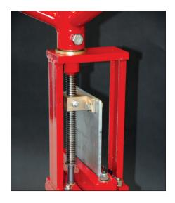
The DX Valve with non-rising stem is available in sizes 3" - 24" and is provided with standard handwheel mechanisms featuring fabricated aluminum tubular handwheels. Gear operators as well as pneumatic and electric operators are also available.
