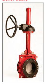
Bevel gears are recommended for high-pressure service or larger diameter valves. Suggested on all DX Valves over 6" in diameter and above 75 psi working pressure.
