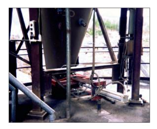
A portable hydraulic power unit can be specified to actuate the DX Valve. A transportable unit is especially convenient for actuating valves in out-of-reach or inconvenient locations, such as tailing lines. Also common is the use of one portable hydraulic unit to actuate multiple valves in close proximity, as found at a cyclone separator.
