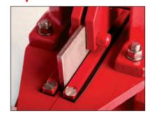
A wiper blade mounted on the top of the valve prevents the gate lubricant and process from leaking through the top. The DX Valve design eliminates the need for traditional packing. This wiper blade also prevents external grit from entering the valve body.
