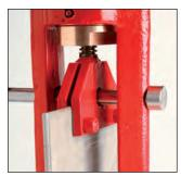
The Series DX incorporates a double pin clevis-to-gate assembly designed to overcome excessive torque, tension and compression forces typically found in heavy slurry applications. This design distributes forces from clevis to gate preventing gate pull-through when opening and binding while closing.
