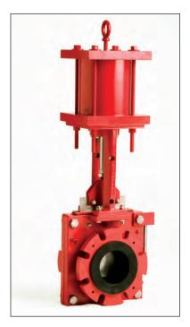
Red Valve manufactures its pneumatic cylinder actuators with a fiberglass-reinforced epoxy resin. The cylinder material is inert to most corrosive chemicals, hydraulic fluids, water and oil. It has an operating temperature range from -90° F to 225° F and can withstand maximum working pressures of 250 psi. Inside actuator walls are polished and impregnated with molydisulfide for reduced friction and wear.
